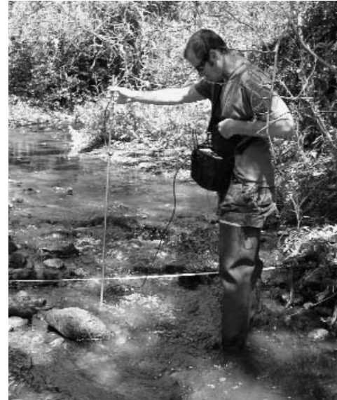
A volunteer measures the flow of a healthy Morro Bay Watershed creek.
