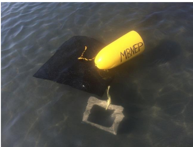
Figure 16. The test seed-bag design: cinder block, attached to oyster bag, attached to a buoy.
