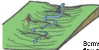
Berms used to slow water flow and create mini-retention basins in a small valley.
