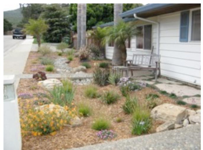
**Rain garden** captures and infiltrates rainwater from a roof in Los Osos, CA. Roof downspouts discharge runoff to vegetated areas.
