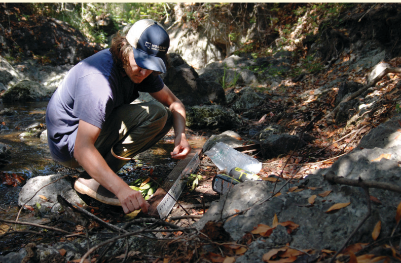
An Estuary Program staff member prepares instruments for installation in Pennington Creek to track creek water levels.
