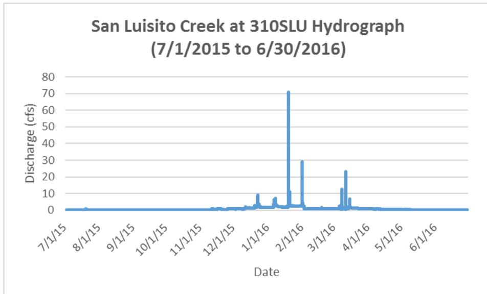
Figure 1 shows discharge (cfs) from July 1, 2015 to July 30, 2016 on San Luisito Creek on Adobe Road. Discharge values were calculated using stage heights from the SLO County FC & WCD stage recorder and the rating curve outlined in previous sediment reports.
