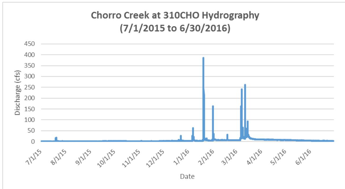
Figure 2 shows discharge (cfs) from July 1, 2015 to July 30, 2016 on Chorro Creek at Canet Road. Discharge values were calculated using stage heights from the SLO County FC & WCD stage recorder and the rating curve outlined in previous sediment reports.
