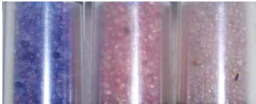
Desiccant stages from left to right: new (left); nearly expired, should replace now (center); expired (right).
